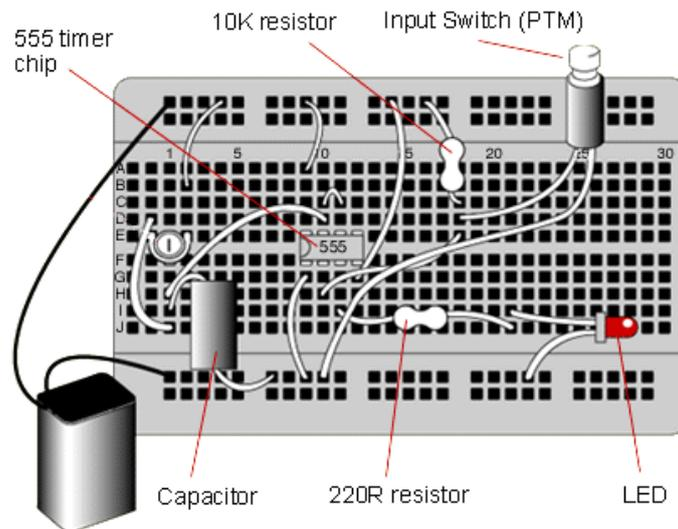
Breadboards are a **temporary construction** method, meaning components are not permanently attached so it is still easy to move them around or to replace them in order to evaluate possible improvements to the circuit.
