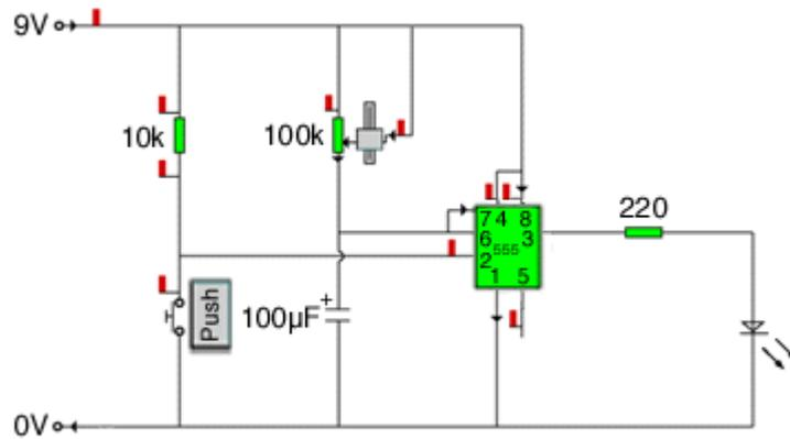
Once the circuit diagram has been created, CAD software can use this to create the design for the printed circuit board, which is much quicker than doing it manually.
